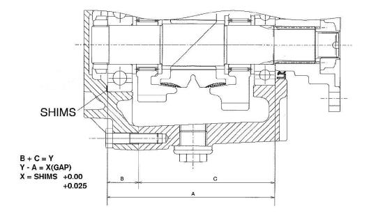
Place the Shims into the appropriate bore of the Front Cover (1) so that they are located under the Bearing (33). Locate both Input and Idler Shaft assemblies into the respective bores. Fit the two Dowels (27) and apply silicon sealant onto the joint face. Tighten the gearcase joint to the recommended torque (see torque chart 10.2). Fit Locknut (25) to the Idler Shaft (7), tighten to the recommended torque (see torque chart 10.2).
