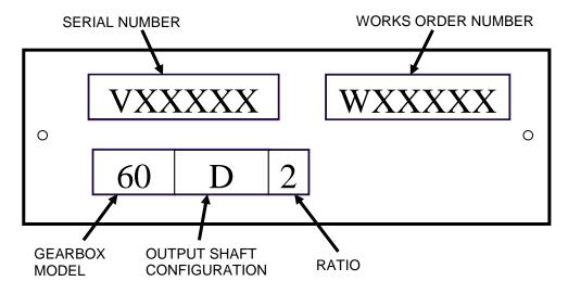
Figure 1 - Example of Serial Plate
