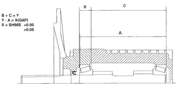
Place the Shims into the appropriate bore of the Front Cover (29) so that they are located under the Bearing cups (25).
