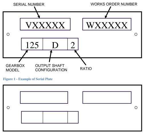
Figure 2 - Blank Serial Plate
