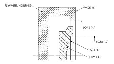
**Figure 3 - Checking the Flywheel and Flywheel Housing**
